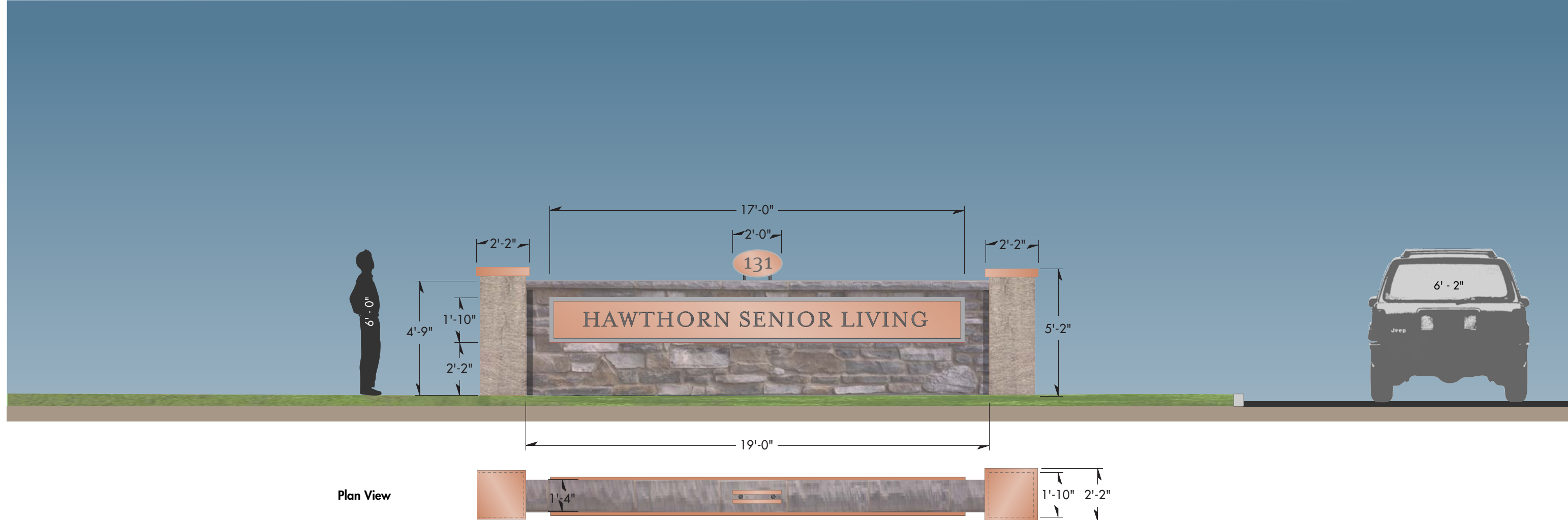
RID 3 Hawthorne ID Elevation & Plan at building Scale: 1/4" = 1'-0"
