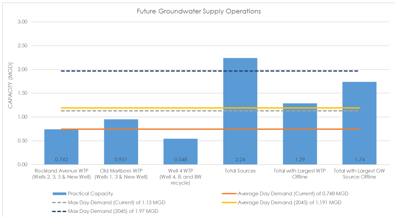
Figure 2 – Future Capacity with Groundwater Source Improvements & OMR WTP Treatment Upgrades
